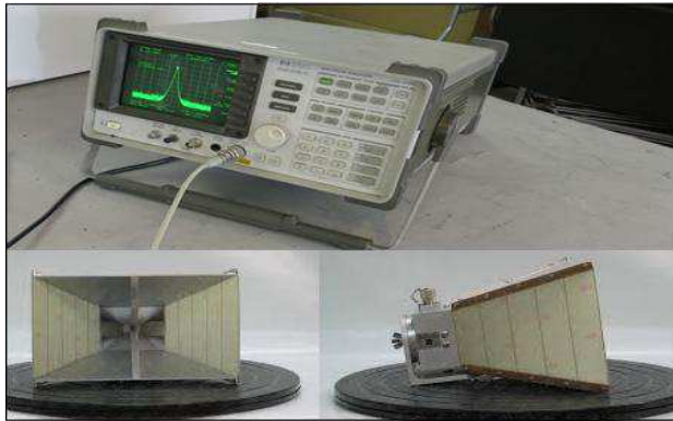
Figure 1. Double-ridged waveguide horn antenna with spectrum analyzer
